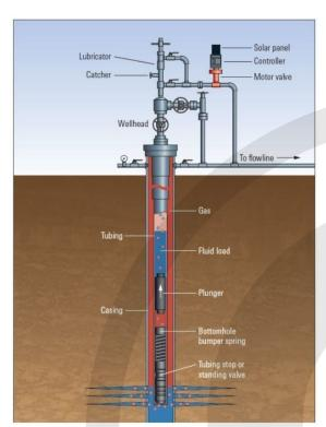
An optimized plunger lift well is achieved when the well is operating at the maximum number of cycles possible with the energy available and at the lowest average flowing bottom hole pressure.
