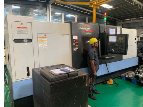
Large Horizontal CNC Milling Machine (Doosan brand)
